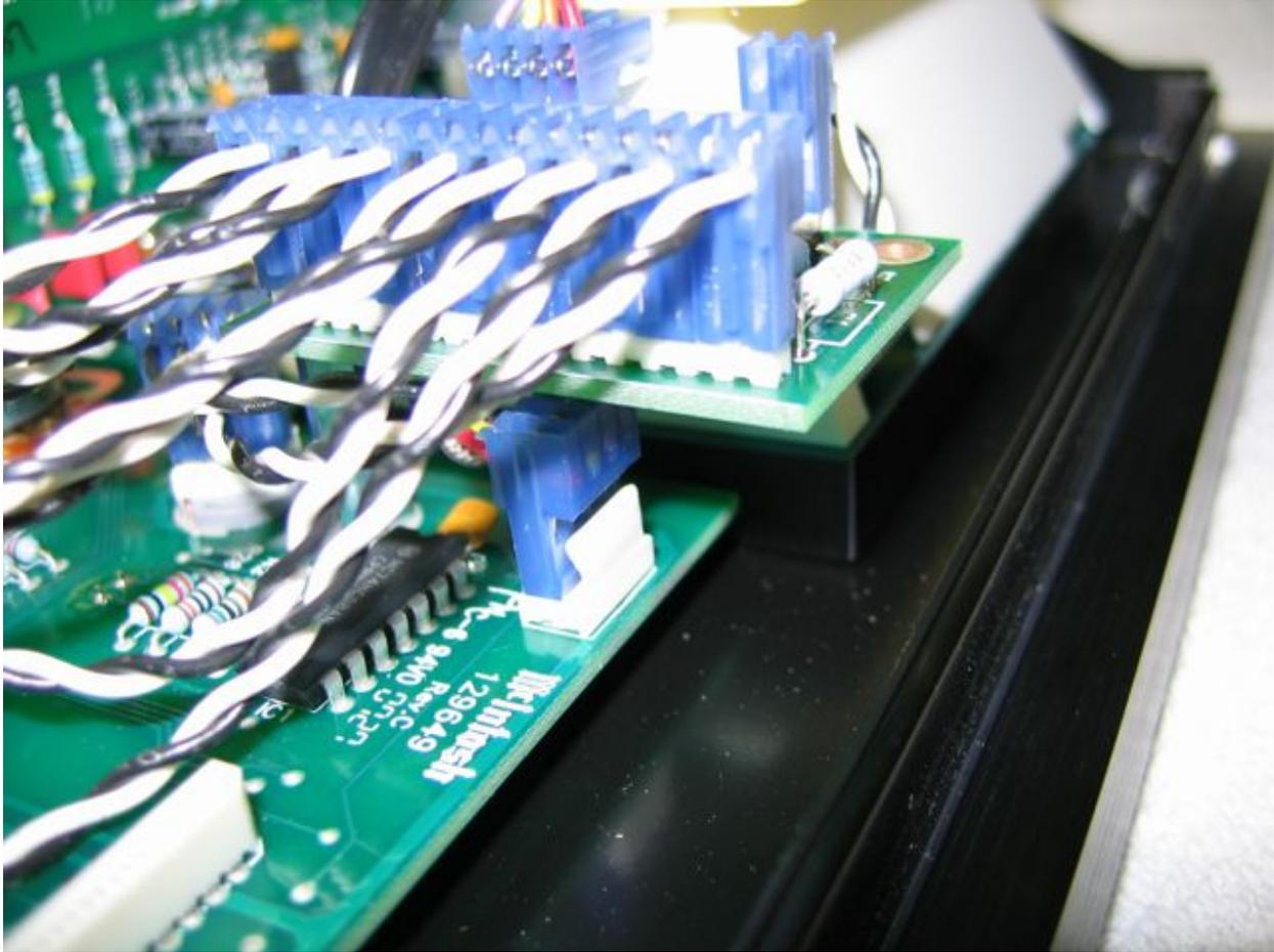
Now remove stock lighting on front panel board, DS15 through DS23 (gray plastic bulb's, eight total) by inserting a straight screwdriver and counter turn 1/4 turn. Replace bulbs with rubber grommet. LED's will insert here as pictured.
