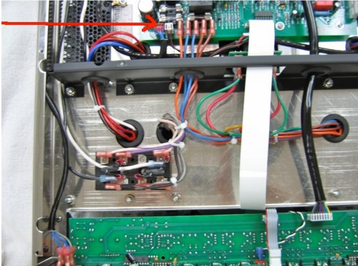
Disconnect the black cable that runs from the front panel to the rear of the unit.
