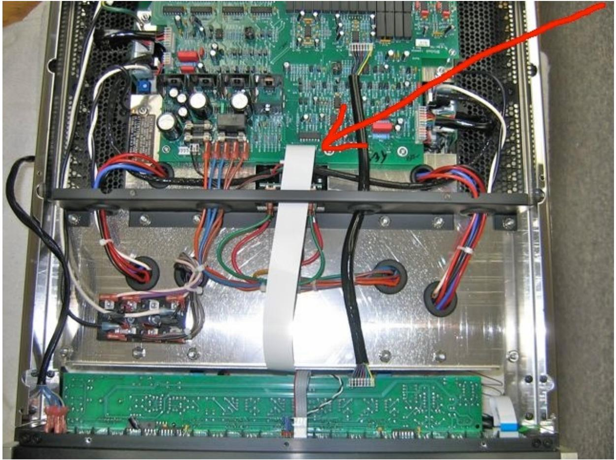
Now remove two black phillips screws on each side that attach the black panel mounts to the stainless chassis.
