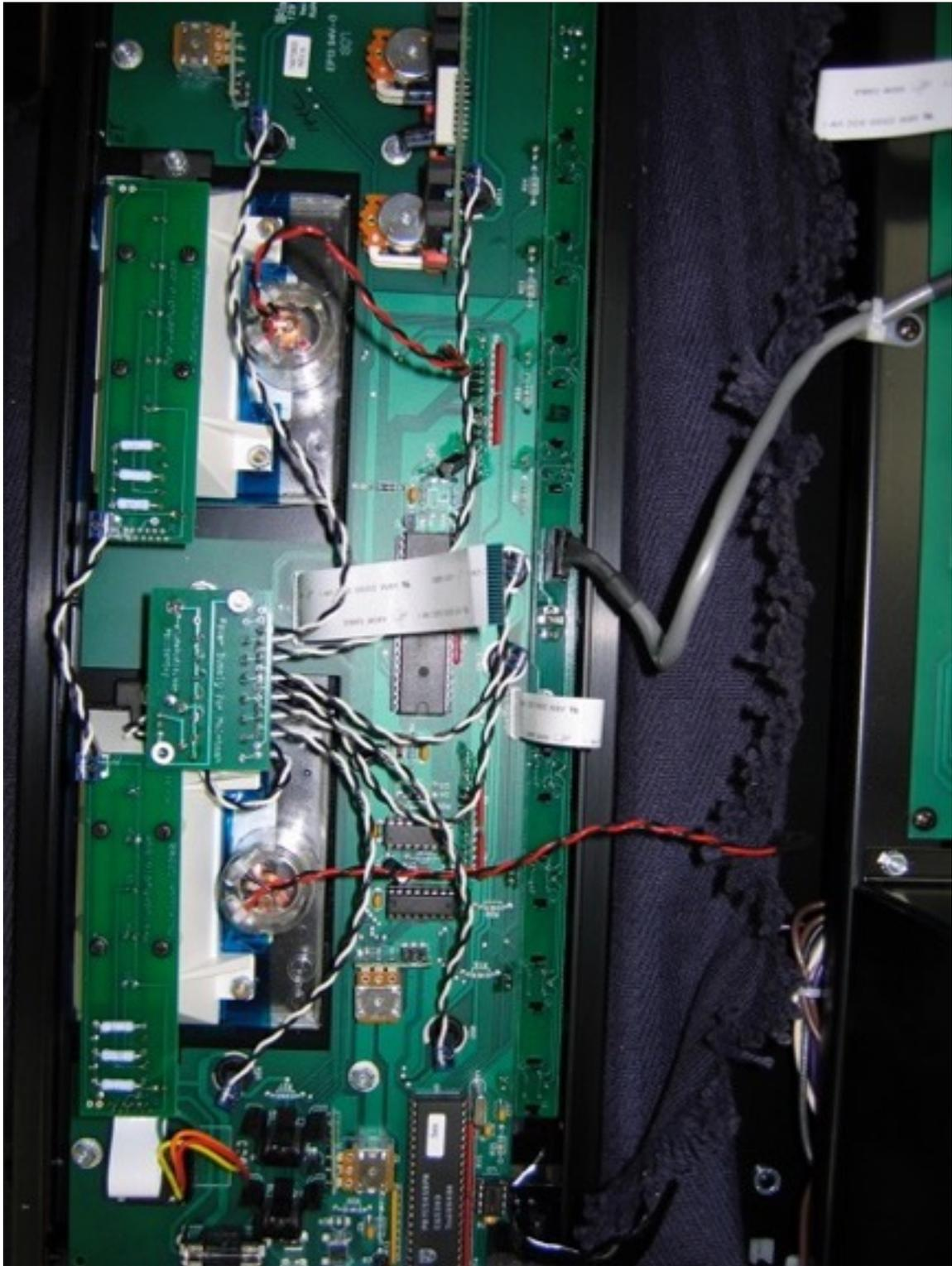
Now mount the revised front panel back on the preamp making sure you attach the Brown wires, the meter wires and all ribbons back into place.
