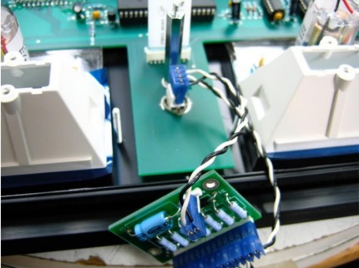
Attach both meter LED assemblies as shown making sure the white ribbon cable is re-attached.
